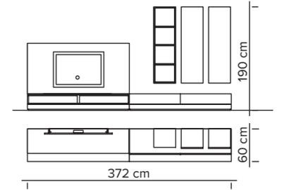
Tidy Novecento panelling is provided with aluminium sections for cables and setting for led lighting installation. The TV holder is supported by brackets and reinforced panels.
